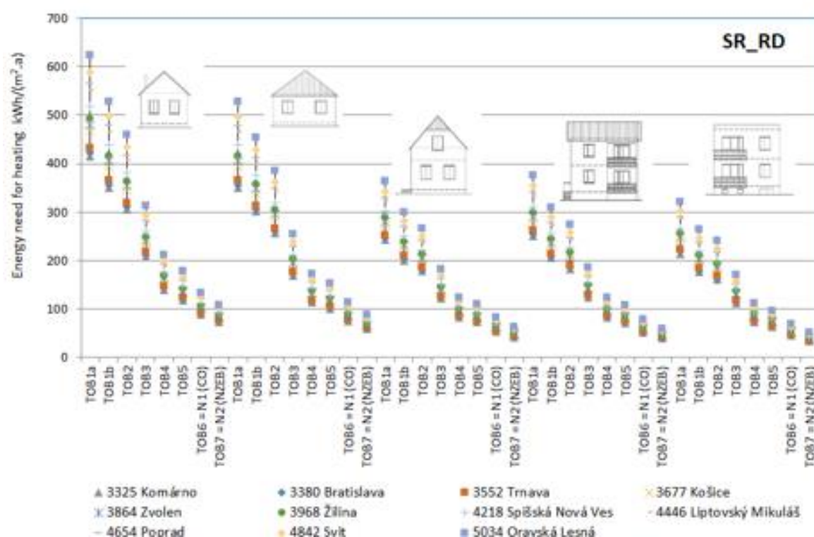
Figure 3-24 Calculated energy need for heating in kWh/(m 2 .a) based on building typology and climate – single family houses
